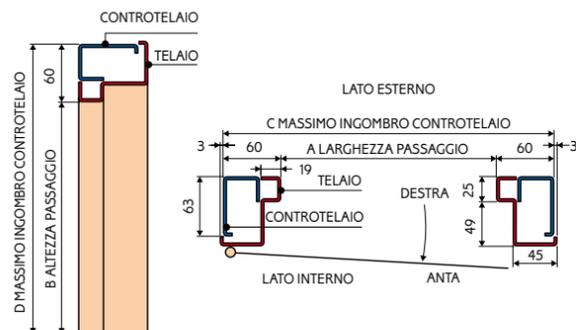
MISURE STANDARD PER IL TELAIO E CONTROTELAIO
