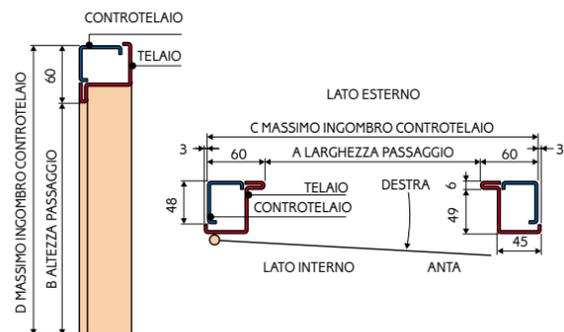
MISURE STANDARD PER IL TELAIO E CONTROTELAIO RIDOTTI
